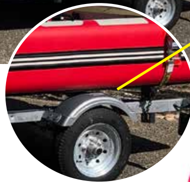
Transom Saver keeps the motor secured at an angle.
