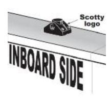
To install the mount, place it over the desired area and drill a 1 3/8" through the fittings at each end of the mount. Be sure the "logo" on the mount reads upright when looking from inboard before securing the mount with the provided hardware.
