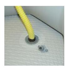
Place the floor inside of the boat with the air valve located in the bow of the boat, facing up. Begin inflating the floor using the high volume setting on the A-50. When resistance is met switch over to the high pressure setting and finish inflating the floor until resistance is met.
