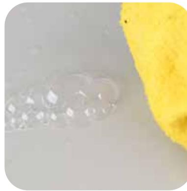
coming from the valve or seams. The leak may produce bubbles, make hissing or sputtering noises, or spray water. Spray bottles are not effective at locating many leaks.
