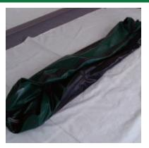
Remove the valve caps and open the valves. Press as much air out of the chambers as possible. First, fold the boat in thirds. Remove seats, etc.
