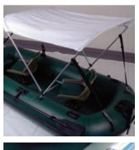
Attach the hardware on the end of the rod when removing the canopy so it is available for next use.
