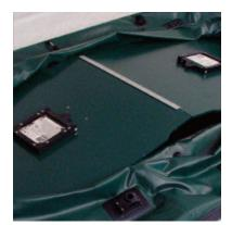
Place the long strut onto the edge of one board. Lift the boards from the middle and insert the edge of the other board into the strut. Press down until fully seated. This step is best done with two people.
