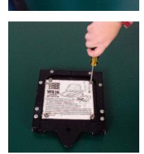
Place the seat mount over the top of the floorboard holes and screw the flathead bolts into the T-nuts.
