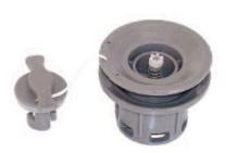
Recessed Air Valves Remove the cap and press and turn the valve stem counterclockwise so that the stem is in the UP position. When the stem is in the up position the valve will retain air. Turning the stem clockwise will put the valve in the down position for deflation.
