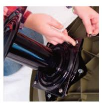
Offset the swivel base so you have enough room to insert the screws and tread the nuts. Tighten the nuts securely.
