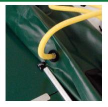
Insert the valve adapter into the valve and turn it to lock the hose in place. If using the foot pump, inflate each chamber until it is very firm. You cannot over inflate with the foot pump.
