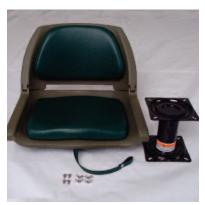
Use the bolts to secure the mounting base to the pads glued onto the boat. Orient the base to the arrow points inboard. Do not use bolts longer than the ones provided as they could puncutre the boat.
