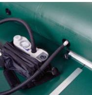
Your STS-10 holds a lot of air. We suggest one of our electric pumps such as the BTP Mano, shown here, to speed the inflation process. While inflating, check that the floorboards are fully seated.
