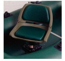
Swivel Seat (OPTIONAL) Slide the base of the pedestal into the seat mount until you hear it lock. To remove, lift the tab and slide out.
