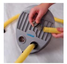
After locating the recessed valve adapter, insert the ribbed end into the hose. We recommend having the foot pump with your boat at all times.
