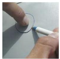
Using a ball point pen, trace the outline of your patch which should be large enough to overlap the damaged area by approximately 1/2". Angle the pen inward a bit so that the ink will be covered by the patch
