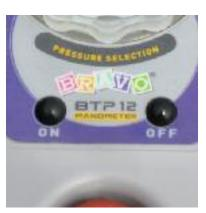
Press the ON button to begin inflation. The pump operates in two stages which can be identified by the noise of the turbine at the start, followed by the piston. The pump automatically stops once the pressure is reached.
