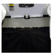
Aft of the boat (at the rear) insert the FB-4 and slide it underneath the transom lip. Exact fit is not critical at this point as the board will be pushed into place when all floorboard pieces have been installed and pressed down.
