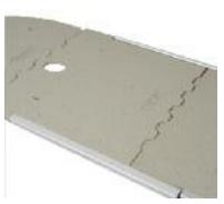
Once both stringers are installed, repeat this process for the opposite side. The second set of stringers should be easier to install with the first set holding the boards in alignment. Once fully inflated the stringers and floorboards will fit firmly into place.
