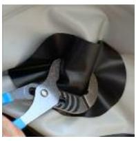
Place the material in the jaws of the channel lock pliers to protect the hull material. Once the body of is unscrewed from the base, pull the body from the opening and insert the replacement. base. The opening is very tight, so you may have to pull on it hard.
