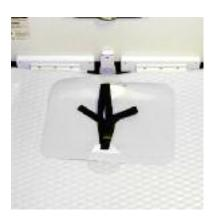
At the stern of the boat near the transom is a fabric guard with buckle and strap to secure a fuel tank.
