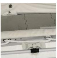
Once deflated, loosen the side stringers with your foot and remove both the stringers and floorboards. You do not need to remove the supports on the FB-2 & FB-4 floorboard pieces. If you have a drop stitch floor, you can deflate it and roll it up with the hull.
