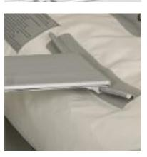
Begin by feeding the fabric beads on the pontoons through the nylon slotted fittings underneath the aluminum bench seat. Slide the seat over the fabric beads so that the seat is toward the center.
