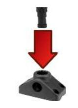
Next, install the rod holder by pushing the post straight down into the mount. Rod holder is designed to enter the mounting bracket only when pointing inboard and is locked in every other direction.
