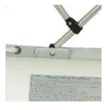
Position the aluminum panel on the outside of the blue material between the front carry handle and the oarlock. and the canopy rods on the inside.
