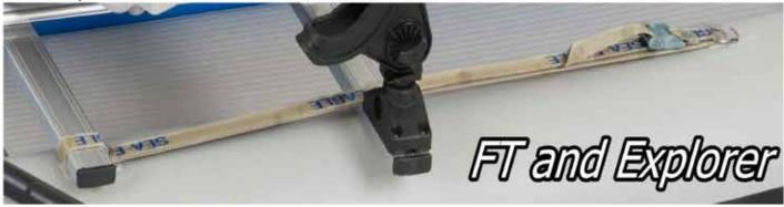
**Tandem** 465FT shown here with optional motor and motor mount. The strap goes under then over the front bar and over the rear rod holder bar. The front D-ring is just behind the bar.
