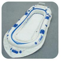
When done chamber #1 should look like this. This is the backup chamber in the event that the main chamber develops a leak.
