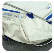
Insert the motor mount bar through the grommets on top of the boat and through the grommet on the bottom. Secure the bottom with the buttons. Repeat with the other rod.
