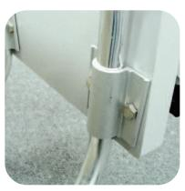
The heads of the bolts should be aligned in the channel on the bracket. The channel is to keep the head of the bolt from turning.
