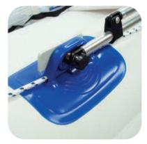
Attach the hardware on the end of the rod. The plate goes inboard. Insert the bolt and washer from inside. Put the brass spacer on the bolt, then rod on the outside, washer and black threaded knob.en down), seat, foot pump and other small items.
