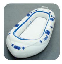
Inflate (the small) chamber, chamber #2 until it is firm. Inflate-chamber #3 while monitoring progress with the Inflation Monitor. Inflate the floor until firm like the other chambers.
