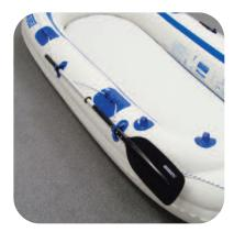
The oars are conveniently stowed on the sides of the boat in clips.
