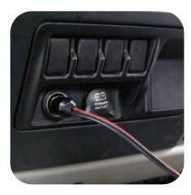
First, check that the pump is switched OFF before inserting the power adapter into your car's power outlet.
