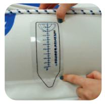
Included with the valves and repair kit is a clear plastic "Inflation Monitor". This 10cm scale is used to determine when the boat has sufficient air.
