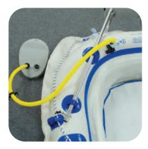
Inflate chamber #1. Insert the hose with the adapter into the valve.
