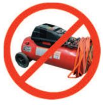
Air compressors that are designed for other uses like tire inflation (usually around 50 PSI) can easily harm your Sea Eagle which has a much lower working pressure. It's for this reason we recommend only using Sea Eagle electric pumps.
