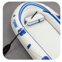
To row your boat using the AB-254 oar set, use the blue carry handles as oar locks. Although the handle is a snug fit for the shaft of the oar, slide the drip ring on the inside of the boat to act as a stopper to keep the shaft in the oarlock.
