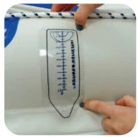
Use the Inflation Monitor to check the inflation progress. When done, the blue Inflation Monitor printed on the boat should match the black scale on the plastic Inflation Monitor.
