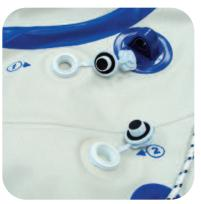
Lay out the boat and place the retainer rings over the valve bases. Stretch the rings if they are too tight to fit overthe base.
