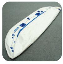
After unscrewing the valves, most of the air should be out, squeeze out any trapped air. Make sure you remove any accessories like the motor mount and bench seats. Fold one side of the boat until it overlaps the floor.
