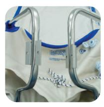
Place the brackets on the rods and adjust them so they are more or less flat to each other. Pro Tip: If you are having difficulty with this step, turn the bracket to one side, slip it on and turn it back.
