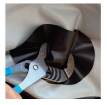
Place the material in the jaws of the channel lock pliers to protect the hull material. Once the body of is unscrewed from the base, pull the body from the opening and insert the replacement. base. The opening is very tight, so you may have to pull on it hard.
