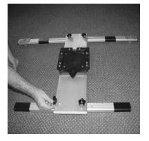
Attach the aluminum board over the 2 yokes at and attach using the 2 long bolts, 2 large washers and 2 black knurled nuts included with the hardware bag. The bolts should be inserted from under the aluminum yoke so the knurled nuts are on top.
