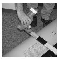
Attach the rod holders through the flush mounts at each end of the long yoke.
