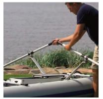
Take one end of each paddle and connect to the extension handles to create the oars. Next, attach the oarlock pins to the fittings at the end of the rowing arm and run the oars through the oarlocks to complete assembly of your rowing frame. Fully tighten the wingnuts before rowing.
