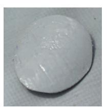
Apply adhesive to the dull side of the patch and around the area to be repaired. Coat the affected area lightly but completely with glue.
