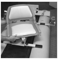
Slide the swivel seat into the quick release seat mount installed on the aluminum board and make sure that the spring loaded mechanism locks it in place.
