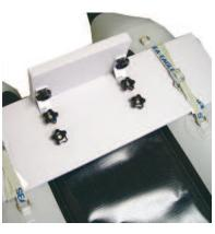
Use the enclosed straps to secure the motor mount board. Run the strap through the Drings fore and aft of the board and tighten. Doing this will pull the motor mount towards the D-Rings fore of the motor mount board.
