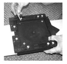
Place the swivel seat mount in the center of the aluminum board and then attach it using the 4 small bolts, washers and wing nuts included with the hardware bag. The aluminum board has 4 pre-drilled holes in the center for this application.
