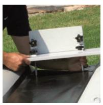
Remove the rear yoke and replace it with the motor mount board which goes over the yoke bolts and secures with the knurled nuts.
