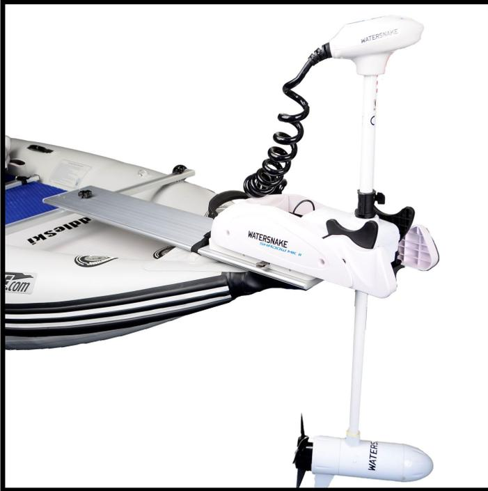
Place motor on quick release and insert locking bar.
