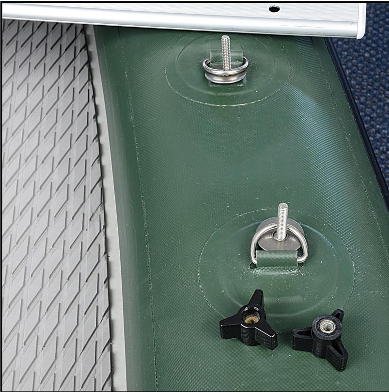
Near the bow (front) of the boat are four D-rings (two on each side) for holding the aluminum board to the boat.
