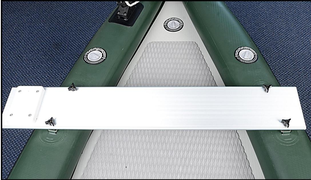
Each FSK16 is hand made so D-ring spacing for each boat is a little different. You may have to push the board back and forth to get the last two bolts through their holes.
