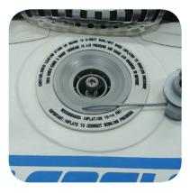
Remove the caps, press and turn the valve stems counterclockwise so that the stem is in the UP position. When the stems are in the up position the valve will retain air.
