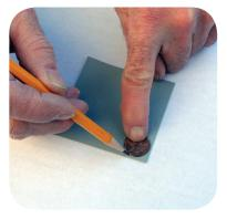
Trace the outline of a penny on the patch material and cut using scissors. Trace the outline of a penny on the boat. Coat the patch and boat with the repair kit glue.
