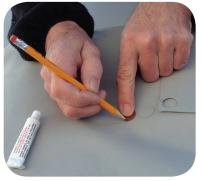
Wait about 5 minutes or until the surface of the glue hazes over then apply the patch. Do not apply wet glue to wet glue.
