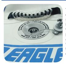
To deflate, push down on the center valve stem and quarter turn it to the right. The stem will stay in the down position, allowing the air to escape. Be sure that your eyes and your face are not directly over the valve.
