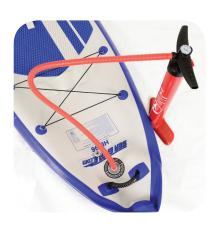
When ready to inflate, insert the adapter into the valve, turn it to the right until it is fully seated and then begin inflation.
