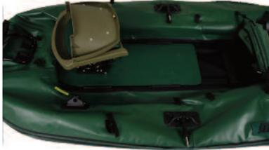
Once the boat loses enough air, remove accessories like oars, motor mount, floorboard seats and rod holders. The mounts for the rod holder can stay on when folding your Sea Eagle.
