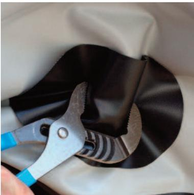
Place the material in the jaws of the channel lock pliers to protect the hull material. Once the body is unscrewed from the base, pull the body from the opening and insert the replacement. base. The opening is very tight, so you may have to pull on it hard.
