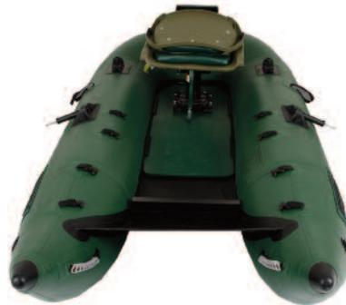
Partially inflate your boat, enough that it takes a bit of its shape. Install the floorboard into the rails making sure that they grip the floorboard. Inflate your Sea Eagle to capacity. For a proper fit, you may have to readjust the floorboard during the inflation period.
