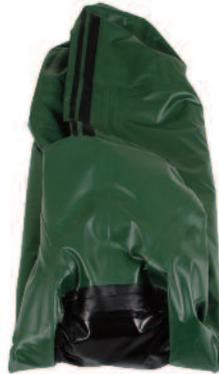
When the excess air has been released you can then fold one of the pontoons over the other and then roll your boat up from stern to bow.
