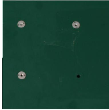
Use the T-Nuts on the bottom of the floorboard when securing the bolts to prevent any abrasion between the bolt and the interior floor.
