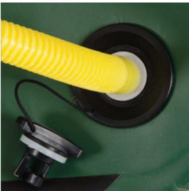
Make sure that the valve stem is in the up position and insert the valve adapter into the valve and turn clockwise to lock into position. Once the desired pressure is reached you should feel resistance on the foot pump.
