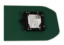
Using the included hardware, attach the seat mount to the predrilled holes on the floorboard. There are 2 sets of pre-drilled holes (6 holes in total). For the best performance we recommend using the first 4 pre-drilled holes closest to the front of the floorboard.
