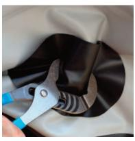
Place the material in the jaws of the channel lock pliers to protect the hull material. Once the body is unscrewed from the base, pull the body from the opening and insert the replacement. base. The opening is very tight, so you may have to pull on it hard.
