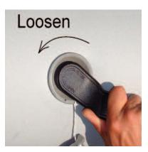
Inflate the chamber to full pressure if possible and loosen with the valve wrench by turning it counterclockwise. Deflate the chamber and unscrew the valve body from the base.
