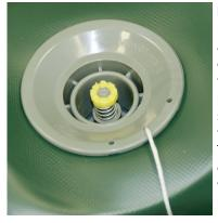
Recessed Air Valves Remove the cap and press and turn the valve stem counterclockwise so that the stem is in the UP position. Only when the stem is in the up position the valve will retain air. Turning the stem clockwise and down will put the valve in the position for deflation.
