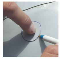
Using a pen, trace the outline of your patch which should be large enough to overlap the damaged area by approximately 1/2". Angle the pencil inward a bit so that the ink will be covered by the patch later.
