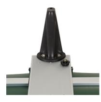
Bolt the raised oarlock bases at both ends of the aluminum bench through the pre-drilled 3/8" holes (2 at each end) using knurled nuts
