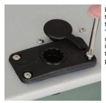
Begin by installing the deck mount onto the bases. Be sure the "logo" on the mount reads upright when looking from inboard before securing the mount with the provided screws.
