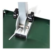
Before attaching the casting bar to your boat, make sure that the FoldCat's pontoons are partially deflated. Insert the upright bases over the underbars in the bow and tighten the set screws at the base using the hex key.
