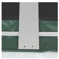
When properly aligned, the underbars should line up underneath the center floorboard. Once they are in place, finish inflating the boat to full capacity.
