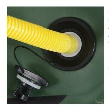
Make sure that the valve stem is in the up position and insert the valve adapter into the valve and turn clockwise to lock into position. Once the desired pressure is reached you should feel a strong resistance on the foot pump.
