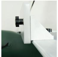
To prevent cavitation when using a short shaft gas motor. The completed setup should hang slightly below the floorboard, as shown. Tighten the knurled nuts and bolts before securing a motor.
