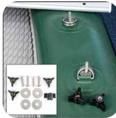
Near valves in bow (front) are four D-rings (two on each side of boat) that hold the aluminum board to the boat. Insert large washer through each bolt. Insert each bolt through a D-ring so it stands upward.
