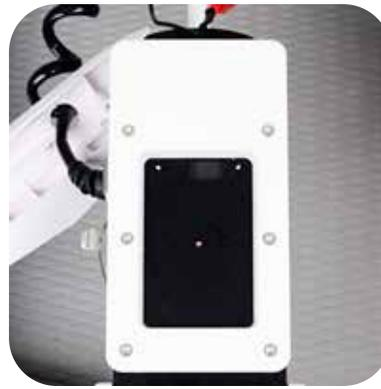
Attach Quick Release base to motor following the video instructions ([Quick Release Bracket](#)). Locking clip must be on the left side when looking at the motor upside down.
