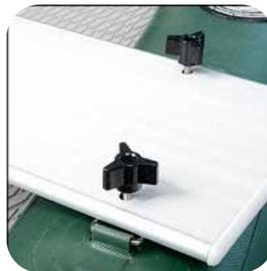
Place board over the bolts on one side of boat and work bolts through the holes. Start threading knobs onto the bolts but do not tighten until bolts are worked through the holes on the other end of the board.
