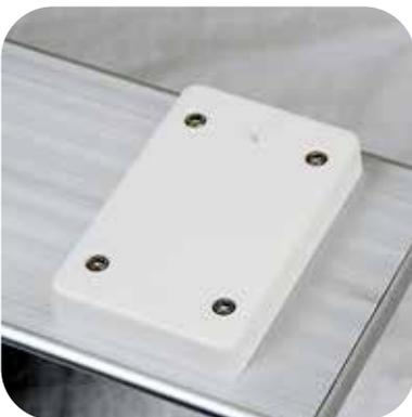
Attach Quick Release adapter block to aluminum board using M6 x 40 mm (1 1/2") socket head screws, washers and locking nuts. The sides are tapered, install so that block and base can slide together.
