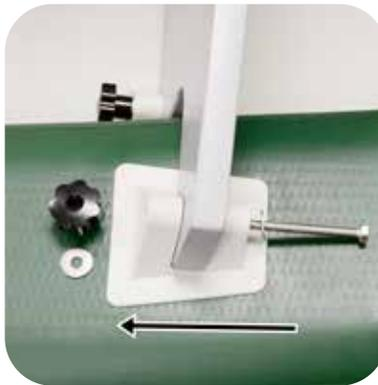
Push the 100mm (4") x M8 bolts with washer through the grommets and transom. If needed, push sides so transom holes align with grommet holes. A wrench is recommended for holding the bolt heads while tightening the threaded knob. When all four bolts are inserted, inflate the side chambers to the working pressure.
