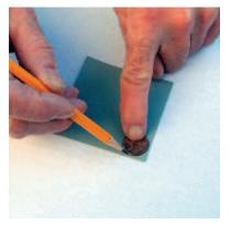
Trace the outline of a penny on the patch material and cut using scissors. Trace the outline of the penny on the boat. Coat the patch and boat with the repair kit glue.
