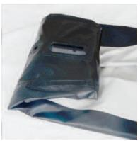
Begin folding from the stern (back) toward the valves. Make the first fold between the end cap and the skeg base. Make the second fold a little past the base, allowing the base to lie flat. A warped base will not allow the skeg to slide in smoothly.
