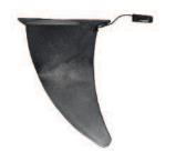
Simply slide the skeg into the skeg base underneath the stern. Then slide the key lock into the small gap in the base to lock it into position. If the skeg will not slide in, do not force it (refer to page 12).
