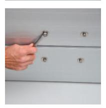
Use the screwdriver to hold the bolt while you tighten the nylock nut with the wrench.
