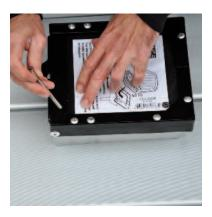
Line up the seat mount on top of the aluminum filler tubes in the center of the aluminum seat board. Once aligned insert the four bolts through the top of the seat mount.
