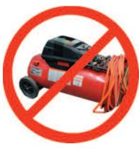
Air compressors that are designed for other uses like tire inflation (usually around 50 PSI) can easily harm your Sea Eagle which works at a much lower pressure of 3.2 PSI. For this reason we recommend
