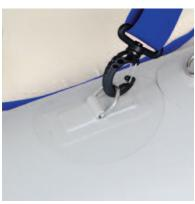
Attach the deluxe seat using the clips on the straps to the D-rings on your kayak. If you're solo paddling, position your seat in the bow of your kayak. For solo paddling, position at the midpoint of the kayak.
