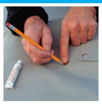
Wait about 5 minutes or until the surface of the glue hazes over then apply the patch. Do not apply wet glue to wet glue. For a demonstration of good patching technique, please view the How to Repair video on the instruction page of our web site. There is a link at the bottom of every page at SeaEagle.com or type "instructions" into the search box.
