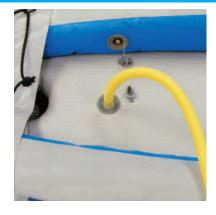
Partially inflate the sides and the floor and check that the floor is tucked underneath the sides. Finish inflating the floor then sides. Working pressure of the sides and floor is 3.2 psi. The floor can be inflated up to 14 psi but is not necessary to do so.
