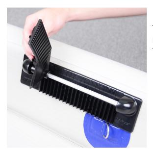
To adjust pedal for comfort and best bracing, raise pedal and slide it along the bar. Note which number the pedal locks at and match it on the other side.
