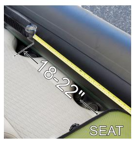
FlexBrace should be installed 18-22" from the front edge of seat base. For Sea Eagle seats, it is the same measurement for DKS inflatable seat but there will be less legroom. This will allow for a wide range of seat and pedal adjustment.
