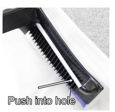
Bend the pad slightly with one hand and push the bar into its hole with the other hand. Inflating the boat will lock the bar in place.
