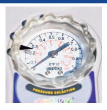
Adjust the pressure dial to read 3.2 PSI which is the operating pressure of your Sea Eagle. PSI is marked in red on the dial. Never turn the dial when the device is under pressure as this will immediately cause the instrument to break.
