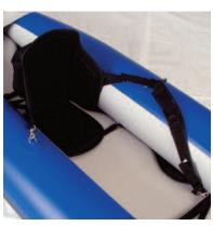
Clip the strap to the floor strap D-ring nearest your feet and clip the other end to the seat D-ring. One strap goes on each side of the kayak. They have an elastic helper that takes up slack when you are not pulling against the strap.
