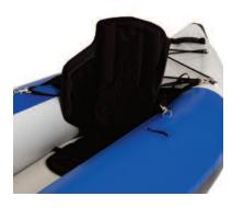
For the rearward seat, clip the back straps to the spray skirt D-rings and the foward straps to the D-rings just in front of the seat. For solo paddling, position at the midpoint of the kayak.
