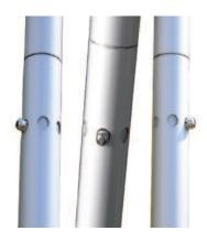
The additional holes in the shaft are for "feathering" the blades. Blades can be offset 45° from each other. This makes paddling into a stiff breeze easier as the blade that is not in the water will be able to slice through the wind with little resistance.
