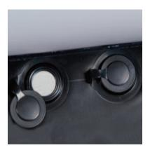
When using the boat in flat-water, screw the caps down tightly. Open the caps before entering whitewater. The boat will partially fill with water when the drains are open.
