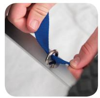
Place the rear of the boat on top of the EZ Cart and run one strap through the eye bolt on each side of the cart. Lay the ends of the strap on top of the boat.
