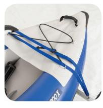
When finished, both straps should be over the top of the boat. The straps can be trimmed if necessary.
