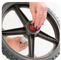
Slide the wheel onto the axle.
