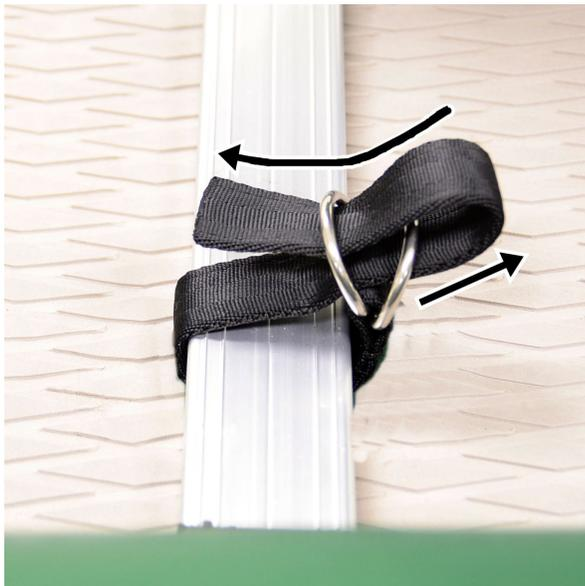
Place the double seat rig over the hold down straps in the FSK16 in either the front or rear position.
