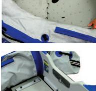
Aft of the boat (at the rear) insert the FB-4 and slide it underneath the transom lip. Exact fit is not critical at this point as the board will be pushed into place when all floorboard pieces have been installed and pressed down.
