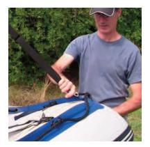
Tie the two rear straps to the back of the boat and then clip the front strap of the canopy to the rope lacing. Keep in mind to tighten the canopy so that it is level and so that it fits tightly on your Sea Eagle.
