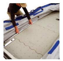
Place the longer stringer in the rear of the boat between the hull and the notched edge of the floorboards with the groove on the stringer ready to accept the edge of the floorboard. Make sure there is enough room for installation of the shorter stringer and insert.
