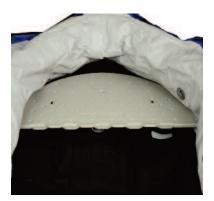
Insert the FB-1 into the bow of the boat. Lift the sides of the boat as necessary in order to slide the FB-1 into place. At this time it does not need to be fully inserted.
