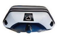
With the floorboard installed and the seat in place, you are now ready to fully inflate the main air chambers of the boat to 100%. If you are using an electric pump, remember to set the pressure to 3.2 PSI before you begin.
