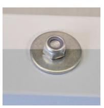
Once the screw is in place, carefully flip the board over and place the small washer and nut over the screw and tighten by hand.
