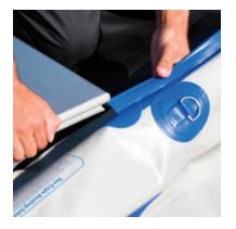
With the boards joined you can now slide the base onto the threaded beads of the boat using the seat hooks located underneath the base. To make installation even easier, partially deflate your FPB and spray/wet the beads before sliding into the seat hooks.
