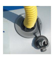
Make sure that the valve stem is in the up position and insert the valve adapter into the valve and turn clockwise to lock into position. Once the desired pressure is reached you should feel resistance on the foot pump.
