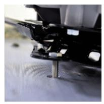
Next, place the swivel seat over the pre-drilled holes at the top and then drop the bolts through the top of the seat and the aluminum boards. Place the large washer over the bolt and secure using the wing nut which you can tighten by hand.
