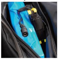
To charge the portable battery, plug it into the charger and then plug the charger into a household electrical outlet. The light on the battery charger will blink red until fully charged. When it is fully charged the light will be a solid green.
