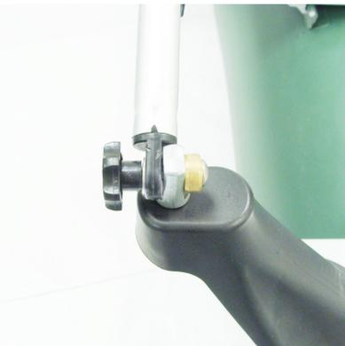
Remove the ring and drop pin into oarlock.
