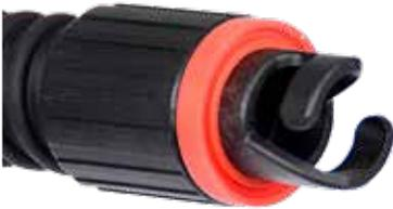
Groove in red gasket must be facing outward. Pull gasket off and reverse it if necessary. Gasket may be stiff upon first use, stretch or kneed gasket to soften it.
