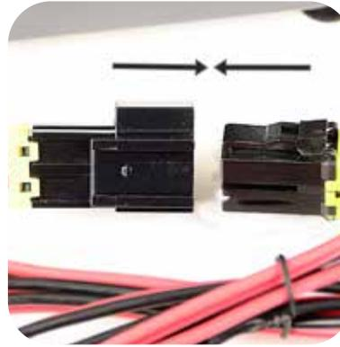
Push wire quick connect into pump quick connect until they click together. To disconnect, press the catch piece on top and pull apart.
