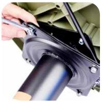
Attach pedestal to seat swivel with the short ½" screws and locking nuts. Hand tighten nuts until all screws have been inserted. Use 7/16" wrench or adjustable wrench to secure the pedestal.
