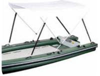
Attach the rear clips to the rear carry handles.
