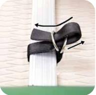
Place frame over the floor straps in the boat. Run strap through both rings (lower arrow in photo). Then run stap back through first ring.
