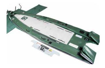
Begin by folding the extensions in half. Keep folding toward the valves and pushing air out.
