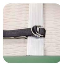
Pull strap tight. Continue securing bar with remaining straps. Check that all are tight.
