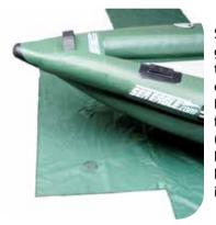
Spread boat bag on the ground. Pull boat over the bag so it overhangs edge of bag by about 4". Remove transom, seat frames, Scotty accessories (but not the screwed-in base), etc. Transom must be removed for boat to fit in bag.
