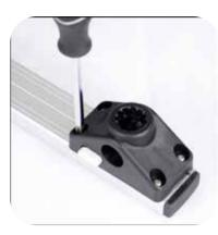
**Scotty Mounts** Use the drill or screwdriver to secure Scotty bases to rod holder bar with #6 x 1 stainless steel screws. Place base so "Inboard" arrow and release button point
