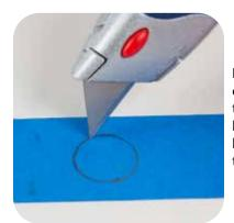
Pro Tip: Trace the outline of the penny on masking tape and cut with a utility knife. Apply tape to the boat instead of tracing on the boat. Sea Eagle offers a large array of accessories for your FishSkiff 16.
