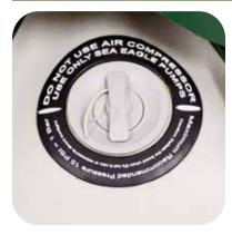
Using the Recessed Valves: Remove the cap to access the valve stem.
