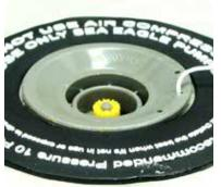
To deflate, push down on the valve stem and quarter turn it to the right. The stem will stay in the down position, allowing the air to escape.
