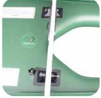
Starting with the floor grommets, insert bolts with flat washer through grommet and transom.
