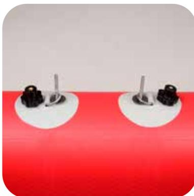
Locate seat hold down D-rings which are attached to sides of boat. Insert M6 x 50 screw with washer through each ring and fold ring flat with bolt pointing upward.
