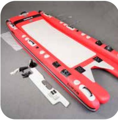
Remove transom, crossbenches, rod holders, and canopy. Rod holder bases remain in place. Place the boat bag under front of boat. Place bag so bottom panel is even with front end of boat and bag is 6 - 8" off center. Push air out.
