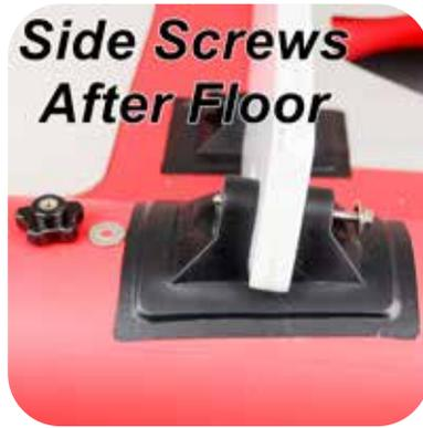
Insert screws with washer through the side chamber grommets and transom holes
