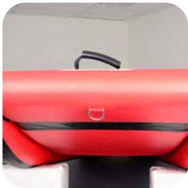
The FastCat12 has a large D-ring located under the front chamber. The D-ring can be used as an attachment point for a trailer winch or to hook up to a mooring.
