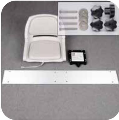
Locate aluminum cross bench(es), quick disconnect seat mount (s), seat(s) and hardware.
