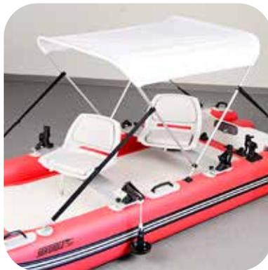
Attach the rear clips to the small D-rings behind transom. Attach front straps behind the front carry handles. Adjust and tighten straps by sliding the buckles.
