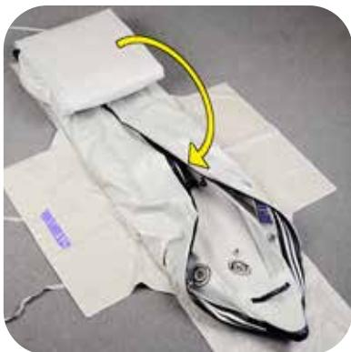
Squeeze air out of the boat. Fold again, this fold will fall on the side-flap of the bag.
