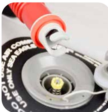
The pump hose has a Recessed Valve Adapter at one end. When ready to inflate the boat, push adapter firmly into valve and twist clockwise to lock in.
