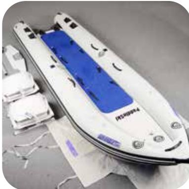
Remove transom, seats, yoke bar, rod holders, and canopy. Rod holder bases remain in place. Place boat bag under middle of boat.
