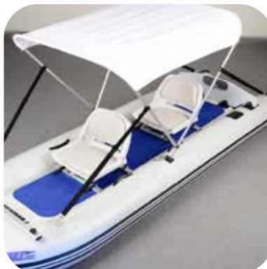
Attach the rear clips to the small D-rings behind transom. Attach front straps behind the yoke bar. Adjust and tighten straps by sliding the buckles.
