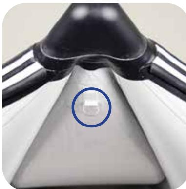
The PaddleSki has a small D-ring located under the front chamber. The D-ring can be used as an attachment point for a trailer winch or to tie up while at the beach.
