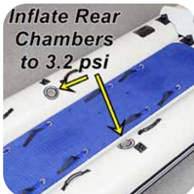
When transom is installed and all screws tightened, inflate the rear chambers.
