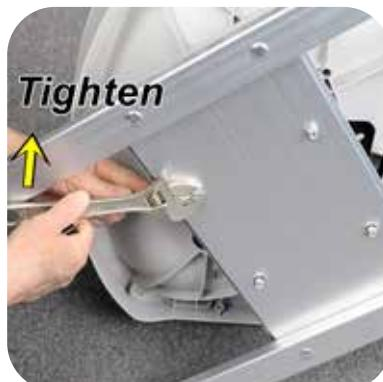
Pull frame up to the screw so it goes through one of the holes. Thread nut onto screw hand tight. Insert the remaining screws and hand tighten the nuts until all four screws are started. With two wrenches tighten locking nuts.
