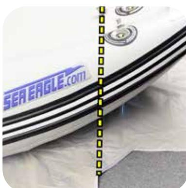
Align the front edge of the bag side flaps with the valves as shown.
