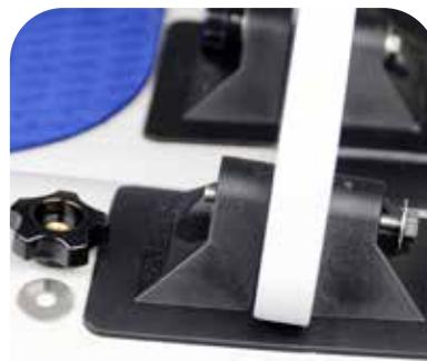
Look through the grommet hole to check alignment with hole in transom. Pull or push bottom of side chamber until holes line up.
