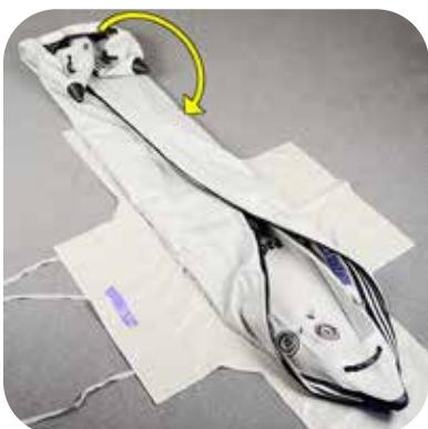
Fold the boat from the back (stern) towards the valves in the front (bow). Make a crease in the fabric about 3-feet from the end between the transom mounting grommets and the rod holders. Make the first fold on the crease.
