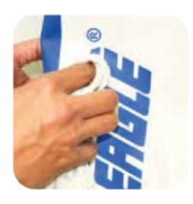
Make sure to thoroughly clean the area surrounding the leak of any dirt or grime. After the area is clean and dry circle the area to make locating the leak easier throughout the repair process.
