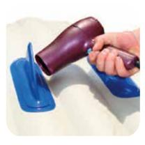
Using a hair dryer, warm the skeg until the curve becomes soft & pliable. This should only take about 2-3 minutes on a normal setting. Once the skeg(s) is soft, you can straighten it with your hands.
