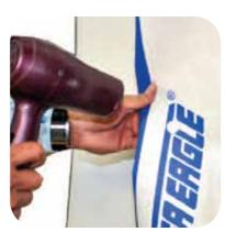
Use a hair dryer on the high setting to activate the adhesive and then press firmly on the patch until it cools.
