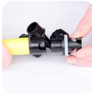
To inflate boat, insert recessed valve adapter into hose. Push adapter in hose and twist to lock.
