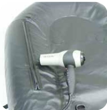
There are four tracking strips on the bottom of the boat which help to maintain course. The tracking strips are very flexible but if they become deformed, heat with a hairdryer until they return to their original shape (1-3 minutes).
