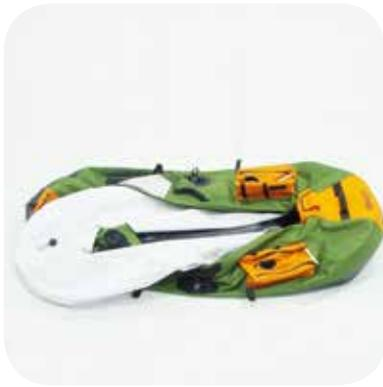
To inspect the air bladder, deflate the boat and pull the bladder out the zipper opening.
