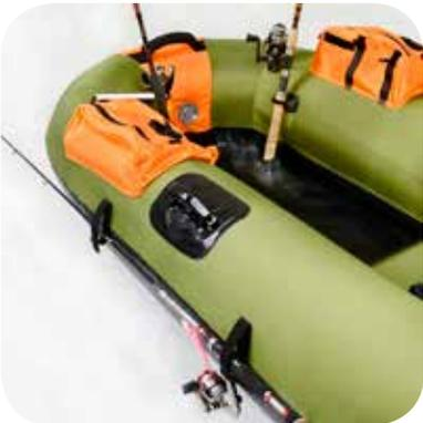
Two fishing rod can be carried in holders located in the front of boat. Two rods can be carried in the hook & loop closure straps on boat sides. Make straps go between the pole and line so rod cannot slip out or loop.
