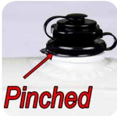
A common error is to pinch the retainer ring between the valve body and base. Trapping the ring breaks the air tight seal. If excess material covers the groove, the ring will go over if stretched slightly.
