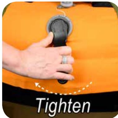
If you suspect a valve is loose, inflate boat to full pressure, insert tool in valve and turn clockwise. Valve has a base which is inside the chamber. Inflating boat will hold base in place while turning valve.
