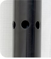
**TIP:** One shaft section has holes for feathering. By feathering the paddle, the blades are offset from each other so that when one blade is in the water, the other is at an angle to slice through the wind with little resistance.
