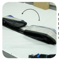
Fold the bow in, then fold the kayak on top of itself. Both nosecones should be folded inside and protected by the kayak walls.
