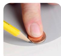
Trace the outline of a penny on the patch material and on the boat. If a larger patch is needed, use a larger item as a template.
