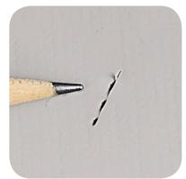
**Patching** The most common repairs are a puncture or small cut. A penny size patch is sufficient for repairs of this type.
