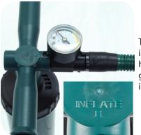
Twist the pressure gauge into "Inflation" port on the handle. Twist hose onto gauge. Inner red numbers indicate PSI pressure.
