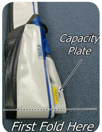
Make the 1st fold at the capacity plate.
