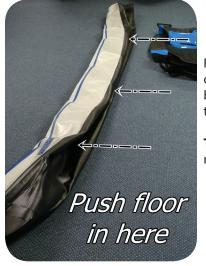
Fold one wall over the other. Push the floor in between the walls for a tight, compact fold.
