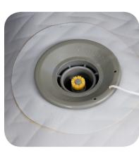
To deflate, push down on the valve stem and quarter turn it to the right. The stem will stay in the down position, allowing the air to escape.
