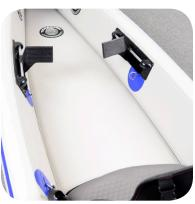
After inflation, adjust pedal for comfort and best bracing, raise pedal and slide it along the bar. Note setting number and match it on the other side.
