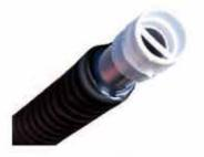
Take adapter number 1 from the cluster and firmly push it into the grey tube in the end of the hose. To ensure that the adapter is fully seated on the tube, push it until the end of the tube pushes past the raised ring in the adapter.
