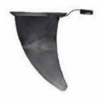
Simply slide the skeg into the skeg base underneath the stern. Then slide the key lock into the small gap in the base to lock it into position.
