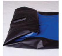
Begin folding from the stern (back) toward the valves. Make the first fold between the end cap and the skeg base. Make the second fold a little past the base, allowing the base to lie flat. A warped base will not allow the skeg to slide in smoothly.
