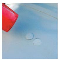
If you have access to electricity, heat the glue with a hair dryer then apply the patch. This method produces the best results.
