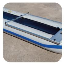
Attach the aluminum tubes that make up the sides of the frame. Orient the bars so the front hole aligns with the mast step bench. Use the 2½" bolt and threaded knob to secure the bar to the bench. Use the 3" bolts to attach it to the middle crossbar.
