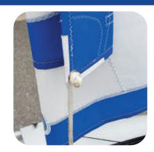
Place the mast with the sail on it into the mast step. Pull the sail down as far as it will go.
