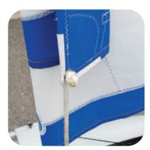
Run the main sheet, the longest and thickest rope, through the grommet in the corner of the sail and tie a knot so it cannot slip through the grommet.
