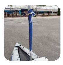
The sail can be furled around the mast without removing the batten. Tightly wrap the sail around the mast. Run the strap through the center of the buckle and out the outer slot. Pull strap tight.
