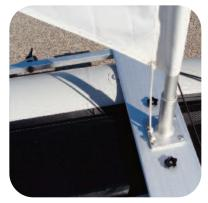
Locate the rope labeled Sail to Mast Step. Tie one end to the corner of the sail and the other end to the loop in the base of the mast step so the sail cannot slide up the mast during use.
