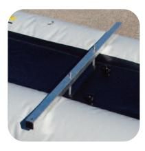
Replace the center yoke bar and bolts with the 36½" tube and the longer (5") bolts included in the kit. If there is vinyl material wrapped around the yoke, remove it now, it is for shipping purposes only.
