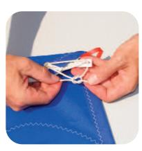
Insert the batten into the opening near the top of the sail. Once it is fully inserted, tie the rope to the fitting.
