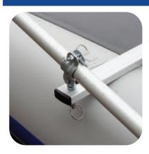
Secure the oar pin underneath the yoke with the ring.
