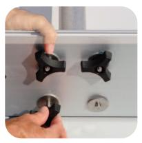
Begin by attaching the mast step to the mast step cross board and secure using the large washers and bolts. For the assembly of the Sail Rig, boat should be only partially inflated.
