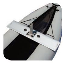
Remove the bow yoke and replace it with the mast step cross board (with attached mast step) and secure the cross board using the yoke bolts and knurled nuts. The loop on the mast step must be facing towards the back of the boat.
