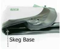
Make the first fold just after the skeg base. Continue folding toward the valves, pushing the air out as you go.
