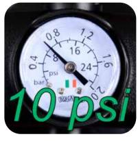
Pump to a working pressure of 7 to 10 psi. Increase pressure depending on weight of passengers and gear or water temperature. Do not exceed 10 psi. (10psi shown in picture.)
