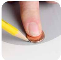
Trace the outline of a penny on the patch material and on the boat. If a larger patch is needed, use a larger item as a template.
