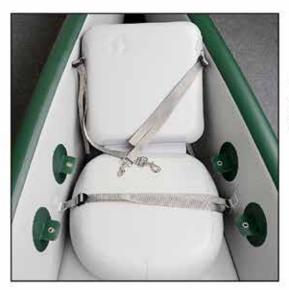
Secure the base with the long strap with buckle. Strap goes up through the center, and down through the front. Pull tight.
