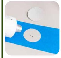
Apply glue to the patch and boat. Allow to dry 15 minutes. Glue must be dry to the touch. If glue layer is thin, apply second coat, allow to dry 15 minutes.
