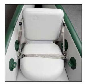
Clip the D-rings to the gray D-rings and pull straps to adjust for comfort.
