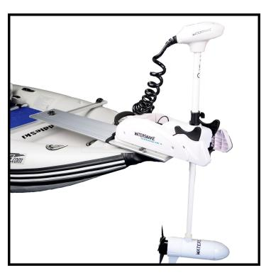
Place motor on quick release and insert locking bar.
