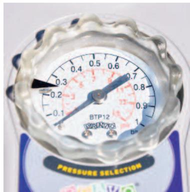
Adjust the pressure dial to read 3.2 PSI which is the operating pressure of your Sea Eagle. PSI is marked in red on the dial. Never turn the dial when the device is under pressure as this will immediately cause the instrument to break.
