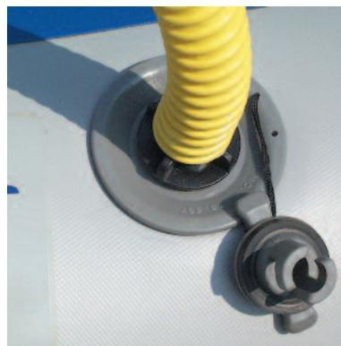
Insert the valve adapter and turn clockwise to lock into position. When the pressure (3.2 PSI) is reached you should feel resistance on the foot pump.
