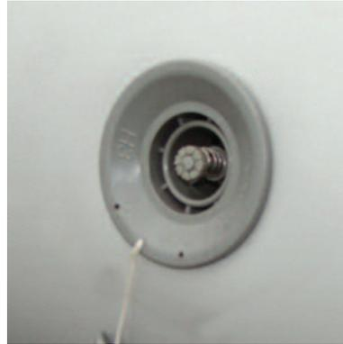
To deflate, press down on the valve stem and turn clockwise to lock into position. Release around 50-75% of the air from each chamber before fully deflating. Excess air can be pushed out as you roll the boat.
