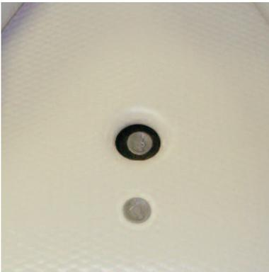
Position the floor for the 10.6SR RIK so that it is located just behind the air valve for the outside drop stitch keel. Inflate the floor first and the keel second. Once the floor is inflated set the A-50 back to the high volume setting and finish inflating the main chambers on the hull.
