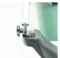
Remove the ring and drop pin into oarlock.
