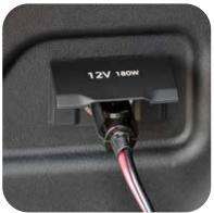
The power connector must be inserted into 12v accessory power outlet. In a vehicle, the 12v power circuit is protected by a fuse, often rated at 10 to 20 amperes (amps). If the pump stops working before inflation is complete, the fuse may have tripped (see troubleshooting).
