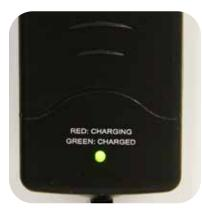
Plug the charger into an outlet (120v). The LED indicator light will show green. Insert the charger wire into the battery charging port 2
