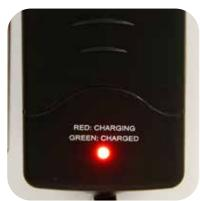
LED will show red when the battery is charging. Charger switches to float (minimum charging) when battery is near full. Light switches to green during float charge. Charging time is usually half-an-hour, but may take three or more hours.
