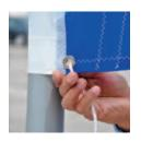
Once the mast is up, take one of the 24" ropes and run it through the grommet on the sail that is closest to the mast.
