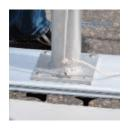
Tie the other end to the loop in the mast step using a double half hitch knot. Secure the rope to the loop on the mast step. Pull the rope tight before tying it off.
