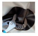
You may need to hold the base from turning. If a tool is needed, place a piece of repair material in the jaws of channel lock pliers to protect the hull material. This is especially true of new boats because the material is still quite soft. Once the valve body is unscrewed from the base, pull the valve body from the opening. The opening is very tight, so you may have to pull hard.
