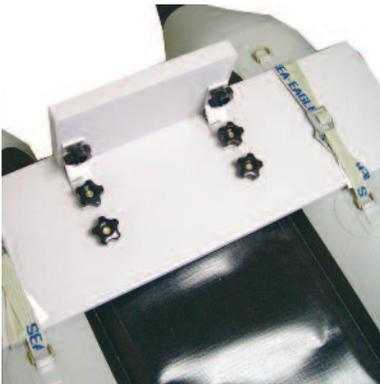
Use the enclosed straps to secure the motor mount board. Run the strap through the D-rings fore and aft of the board and tighten. Doing this will pull the motor mount towards the D-Rings fore of the motor mount board.
