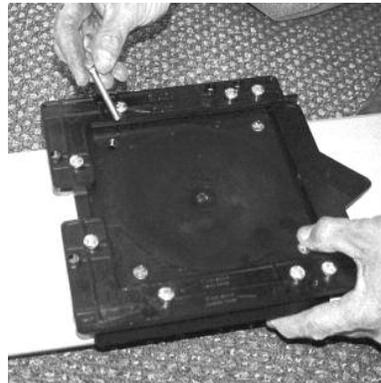
Place the swivel seat mount in the center of the aluminum board and then attach it using the 4 small bolts, washers and wing nuts included with the hardware bag. The aluminum board has 4 pre-drilled holes in the center for this application.
