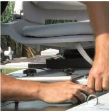
Remove the center crossbar yoke from the PaddleSki, leaving the bolts from the yoke in place. Attach the smaller yoke connected to the assembled frame and secure it to your PaddleSki using the knurled nuts. The longer yoke does not need to be bolted down.
