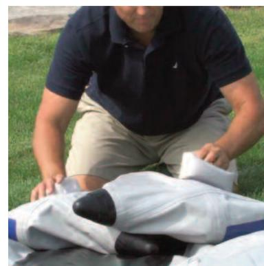
Begin to roll your boat from the stern. Fold the pontoons in and replace the skeg protectors over the skegs. Continue rolling your boat up until you reach the bow and tuck the bow in.
