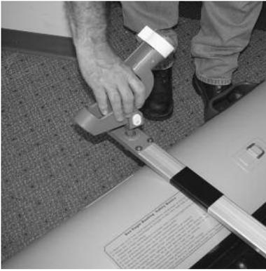
Attach the rod holders through the flush mounts at each end of the long yoke.
