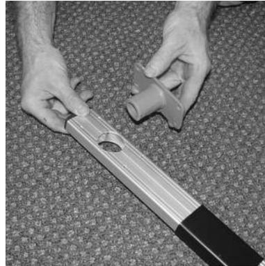
Attach the flush mount adapters for the rod holders at each end of the long yoke in the pre-drilled hole and secure with a Philips Head Screwdriver.
