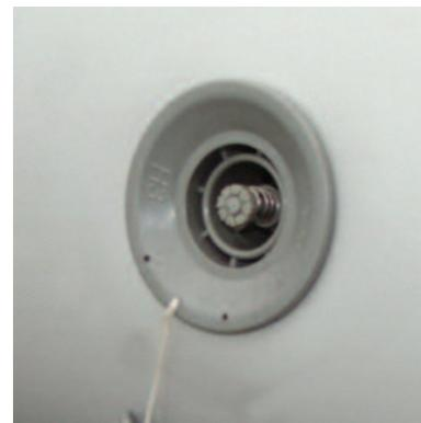
To deflate, press down on the valve stem and turn clockwise to lock into position. Release around 50-75% of the air from each chamber before fully deflating. Excess air can be pushed out as you rollup the boat.
