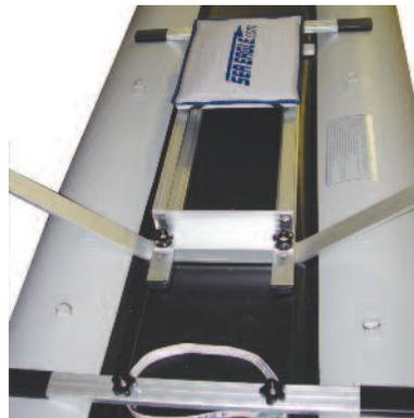
Once assembled, place between the middle and the aft (toward the rear) crossbar yoke. The sliding seat must touch the middle crossbar yoke to prevent movement of the frame while rowing. Loop the included foot strap around the bolts of the aft yoke to lock your feet while rowing.
