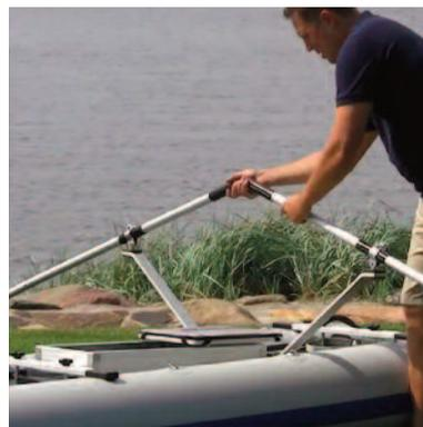
Take one end of each paddle and connect to the extension handles to create the oars. Next, attach the oarlock pins to the fittings at the end of the rowing arm and run the oars through the oarlocks to complete assembly of your rowing frame. Fully tighten the wingnuts before rowing.
