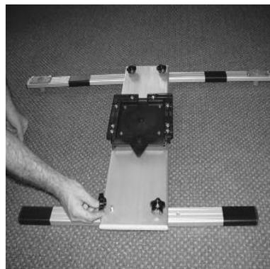
Attach the aluminum board over the 2 yokes at and attach using the 2 long bolts, 2 large washers and 2 black knurled nuts included with the hardware bag. The bolts should be inserted from under the aluminum yoke so the knurled nuts are on top.
