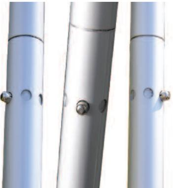
The 3 pre-drilled holes are used for feathering so that you can position one blade to 90° from the other. This makes paddling into a stiff breeze easier because the blade that is not in the water will be able to slice through the wind with little resistance.
