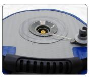
To deflate, press down on the valve stem and turn clockwise to lock in open position. Most of the air is immediately released. Excess air can be pushed out as you fold up the board.
