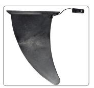
A large removable skeg is included with your NeedleNose for improved tracking. Make sure that the key lock is in the out position of the skeg (as pictured) before sliding the skeg into the base.
