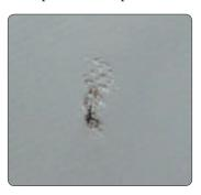
The most common repairs are a puncture or small cut. A penny size patch is sufficient for repairs of this type.
