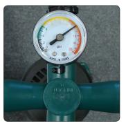
The pressure gauge will not begin to register until the board begins to get pressurized. Pump until the working pressure of between 12 and 15 psi is reached.
