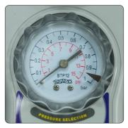
Adjust the pressure dial to read 12-15 PSI which is the operating pressure of your Sea Eagle. PSI is marked in red on the dial. Never turn the dial when the device is under pressure as this will immediately cause the instrument to break.
