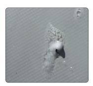
Soapy Water Test Inflate the boat to full pressure. Mix a couple of tablespoons of dishwashing liquid in a bucket of water.
