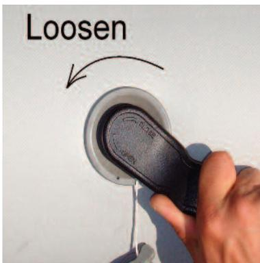
Inflate the chamber to full pressure if possible and loosen with the valve wrench by turning it counterclockwise. Deflate the chamber and unscrew the valve body from the base.
