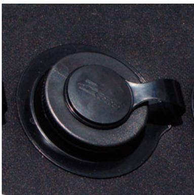
**When using in rapids, tuck the drain valve caps underneath the drop stitch floor. This will make sure that the cap does not interfere with the draining process and still keep the cap readily available to you should you find yourself back on calm, or flat-water.**
