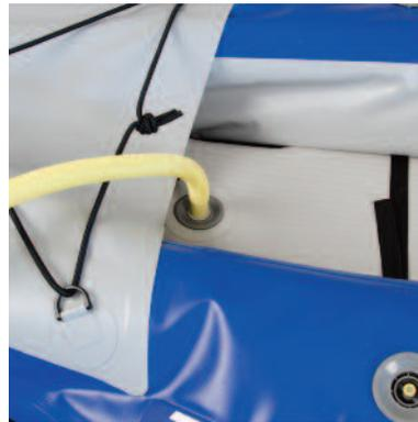
Partially inflate both the side pontoons and drop stitch floor making sure that the opening in the floor is centered with the air valve in the bow and that the floor is tucked underneath the pontoons. Fully inflate the drop stitch floor and then fully inflate the side pontoons.
