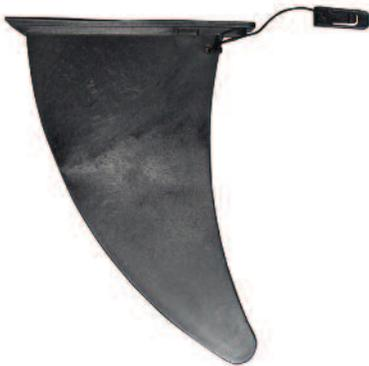
Before installing make sure that the key lock is in the out position of the skeg. Simply slide the skeg into the skeg base underneath the stern and then slide the key lock into the small gap underneath the skeg to lock it into position.
