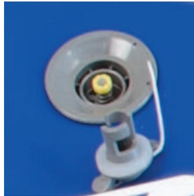
Begin by deflating your kayak. To deflate, press down on the valve stem and turn clockwise to lock into position. Most of the air is immediately released. Excess air can be pushed out as you roll up the kayak.
