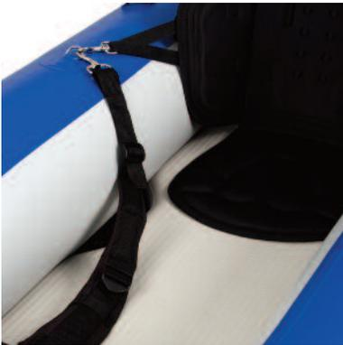
Attach each of end of the thigh straps to the D-Rings at the top of the pontoon and the ones near the floor.
