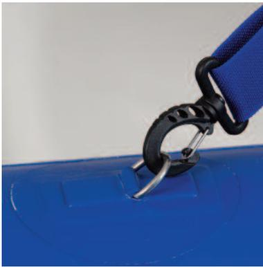
Attach the deluxe seat using the clips on the seat and the D-Rings on your kayak. Adjust the straps on the seat for comfort. If you're solo paddling, position your seat in the bow of your kayak.
