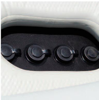
Check the 4 drain valves through the oval cut-out at the stern of your kayak. Make sure the valves are closed tightly if you plan on using your kayak in calm or flat-water. Otherwise open them for drainage if you plan on using your kayak in rapids.
