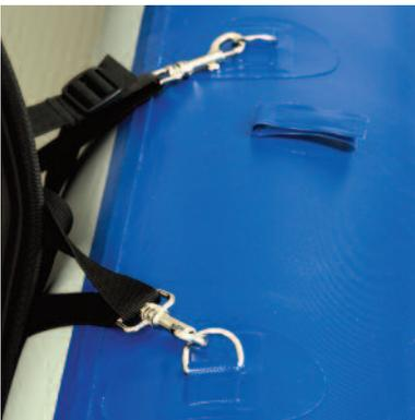
Attach the tall back seat using the clips on the seat and the D-Rings on your kayak. Adjust the straps on the seat for comfort. If you're solo paddling, position your seat in the bow of your kayak and attach the front straps to the first set of D-Rings and the back to the second set.
