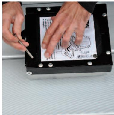
Line up the seat mount on top of the aluminum filler tubes in the center of the aluminum seat board. Once aligned you can then insert the four bolts through the top of the seat mount.
