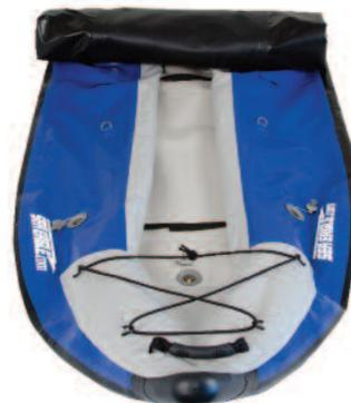
Starting from the stern, roll the kayak up. It is important to roll the boat tight from the beginning to ensure you get the most compact storage possible. When you reach the end, tuck the bow underneath the hull and place inside of the boat bag and secure with the nylon straps.
