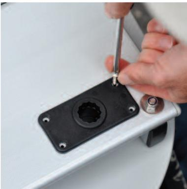
Install the rod holder mount into the platform and secure by tightening the screws with the Phillips head screw-driver.
