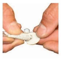
Apply adhesive to the dull side of the patch and around the area to be repaired. Coat the affected area lightly but completely with glue.
