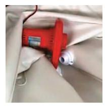
No extra nozzles are needed to inflate the main air chambers of your boat, just insert the pump into the valve and switch it on. Do not drop or suddenly move the pump while it is
