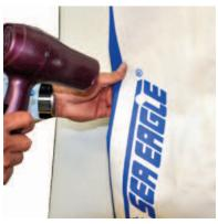
A temperature of approximately 160 degrees will activate the adhesive and from there you can press firmly on the patch until cooled. It is VERY IMPORTANT that you DO NOT use a hair dryer on an inflated boat.
