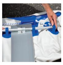
Slide the aluminum motor mount rods through the grommets and the fittings on both the bench seat and motor mount board. Once the rod is installed put the rod pin through the hole at the end of the rod. Repeat this process for both sides.
