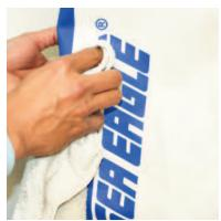
Once you have located the leak make sure you thoroughly clean the area surrounding the leak of any dirt or grime. After the area is clean and dry you can circle the area to make locating the leak easier throughout the repair process.
