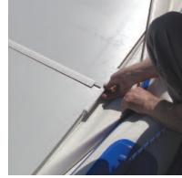
Once the floorboards are in and connected, insert the two small struts on each side of the floorboards where the bow and stern pieces meet.
