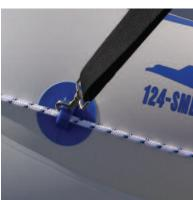
Take the two bow strap on the v-braces and connect it to the grab line on the front grommets on the bow of the boat.
