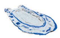
Deflate by unscrewing all of the deluxe oneway valves from the 3 main chambers. You can expedite this process by using the foot pump to suck any excess air out of the boat.
