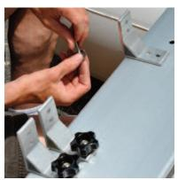
The brackets fasten in two places, the wooden motor mount block and the aluminum motor mount slat. Connect the bracket to the motor mount slat first by taking 1 short bolt & 1 washer and push the short bolt through the bottom of the slat and through the bottom of the bracket.
