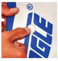
Place the patch on the damaged area and press down firmly. Let the glue sit for 2-4 minutes until it appears tacky. If glue does not hold, heat patch with a hair dryer.
