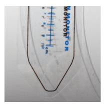
You can safely inflate one centimeter beyond the diagram. Once fully inflated you should be able to indent your thumb into the boat about ½ to ¾ of an inch. If you are using floorboards, only inflate the main chambers 75% full until they're installed and then finish inflation.
