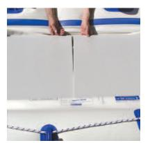
Place both the bow and stern floorboard pieces inside of the boat so that they overlap in the middle.
