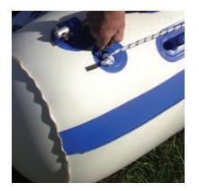
Take the stern strap on the v-brace and connect it to the grab line on the very last grommet on the stern of your boat, repeat this process on the other side.
