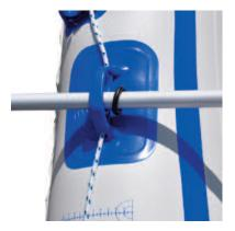
To row your boat using the AB-253 oar set, use the blue carry handles as oar locks. Although the handle is a snug fit for the shaft of the oar, you can keep the drip ring on the inside of the boat to act as a stopper and keeping the shaft in place.
