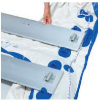
Place the aluminum bench seat between the grommets in front of chamber #1 (behind the rod holders) and then place the aluminum motor mount board (which you can identify by the pre-drilled holes in the middle) between the grommets near the carry handles.
