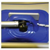
Secure the canopy into position by inserting the bolt through the metal plate. Once through place the brass washer on the bolt and feed the bolt through the side carry handle and secure with the black knurled nut. Make sure that the metal plate is on the inside of the boat.
