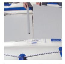
Lift the floorboards and insert the large strut into the center to connect the two pieces. Force the boards down into the boat, being careful not to pinch your fingers or toes in the process.
